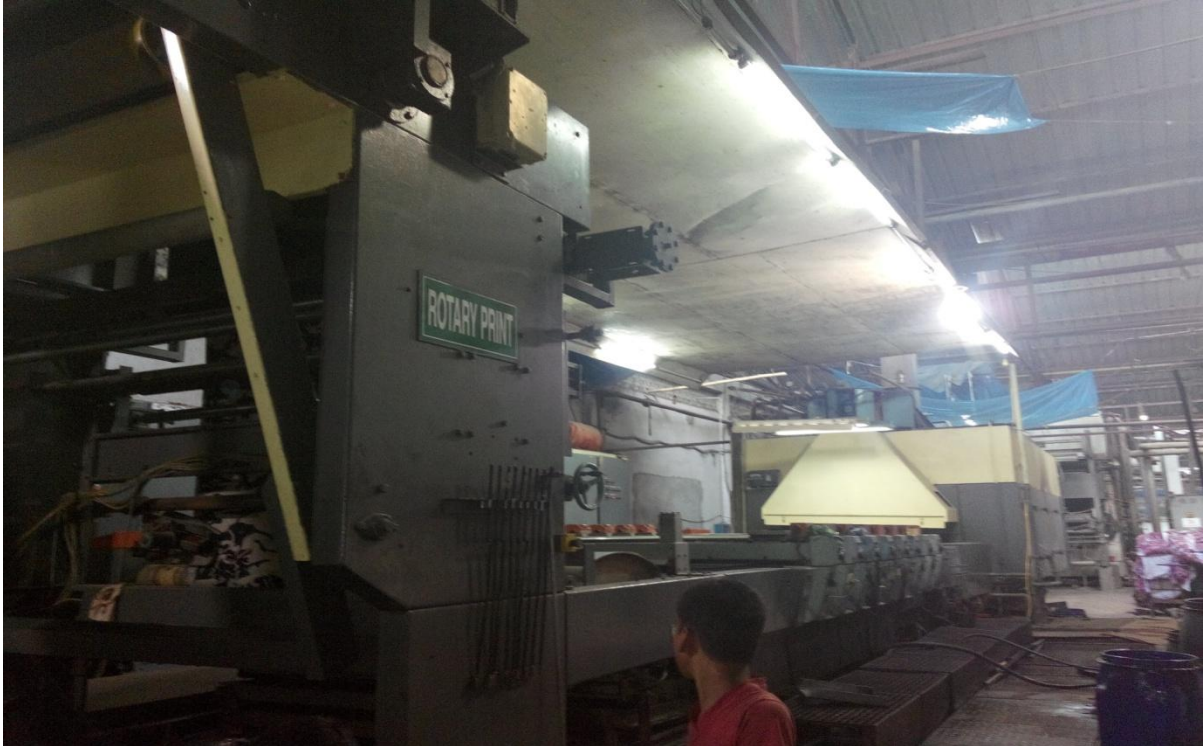
Figure No 12: Pictorial view of Rotary screen Printing Machine.
