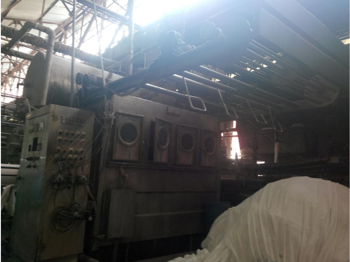
Figure No 07: Pictorial view of Winch Machine.
