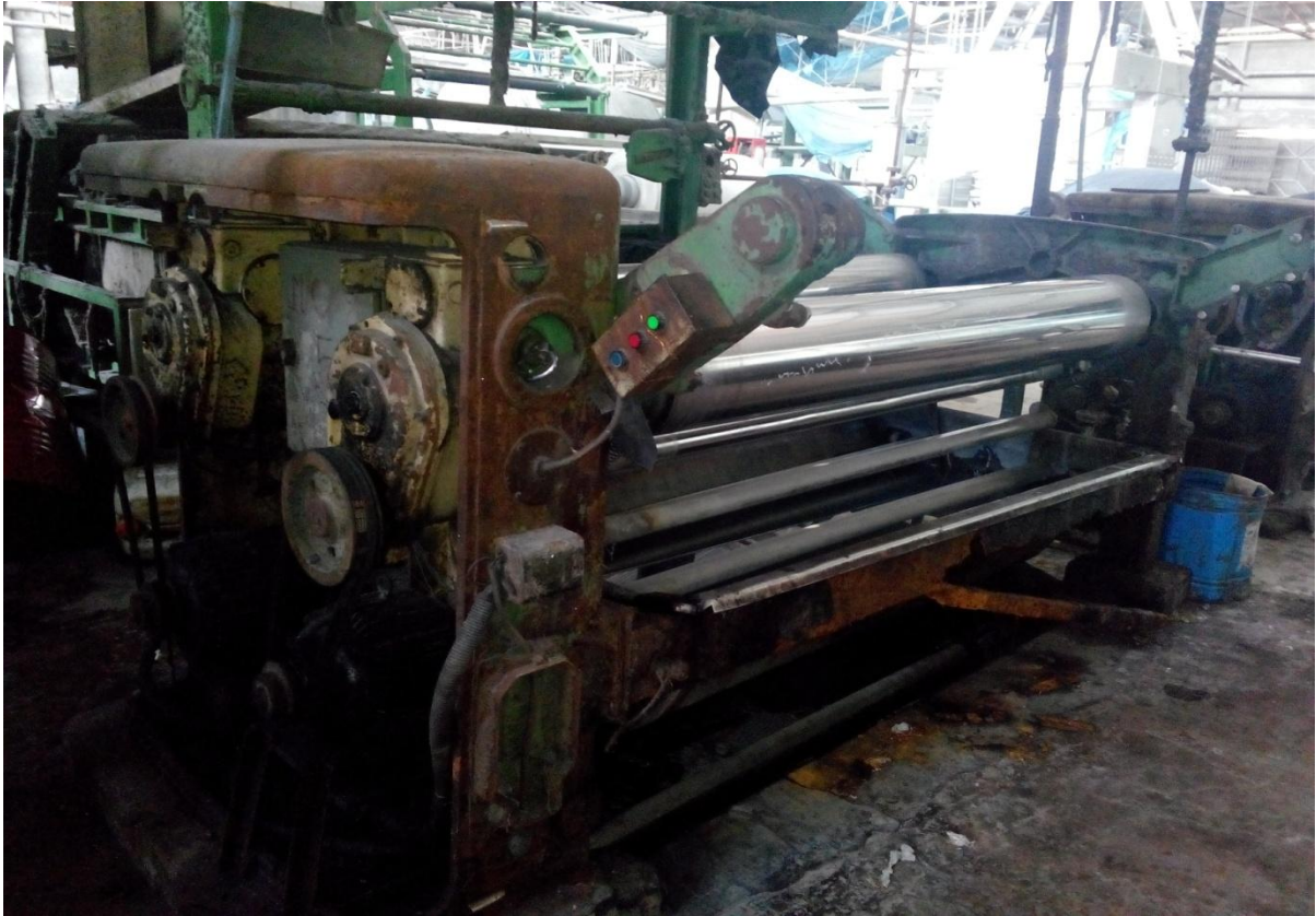
Figure 04: Pictorial view of Jigger Machine.
