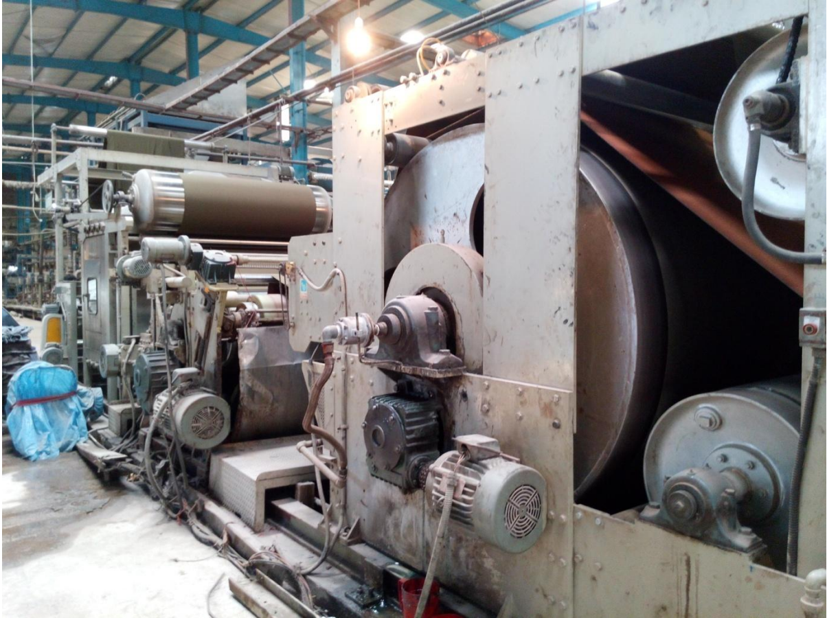
Figure No 10: Pictorial view of Sanforising Machine.
