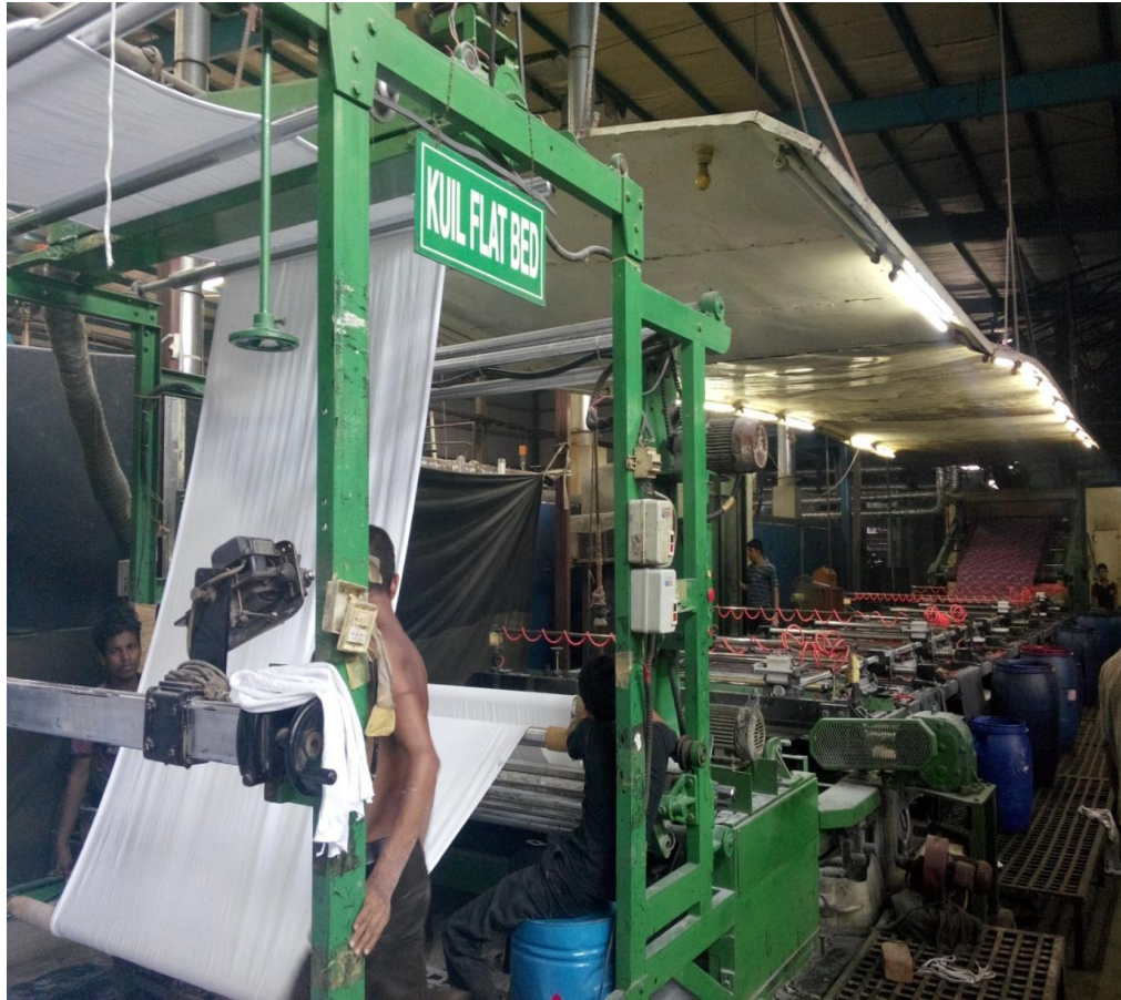
Figure No 11: Pictorial view of Flat bed screen Printing Machine.
