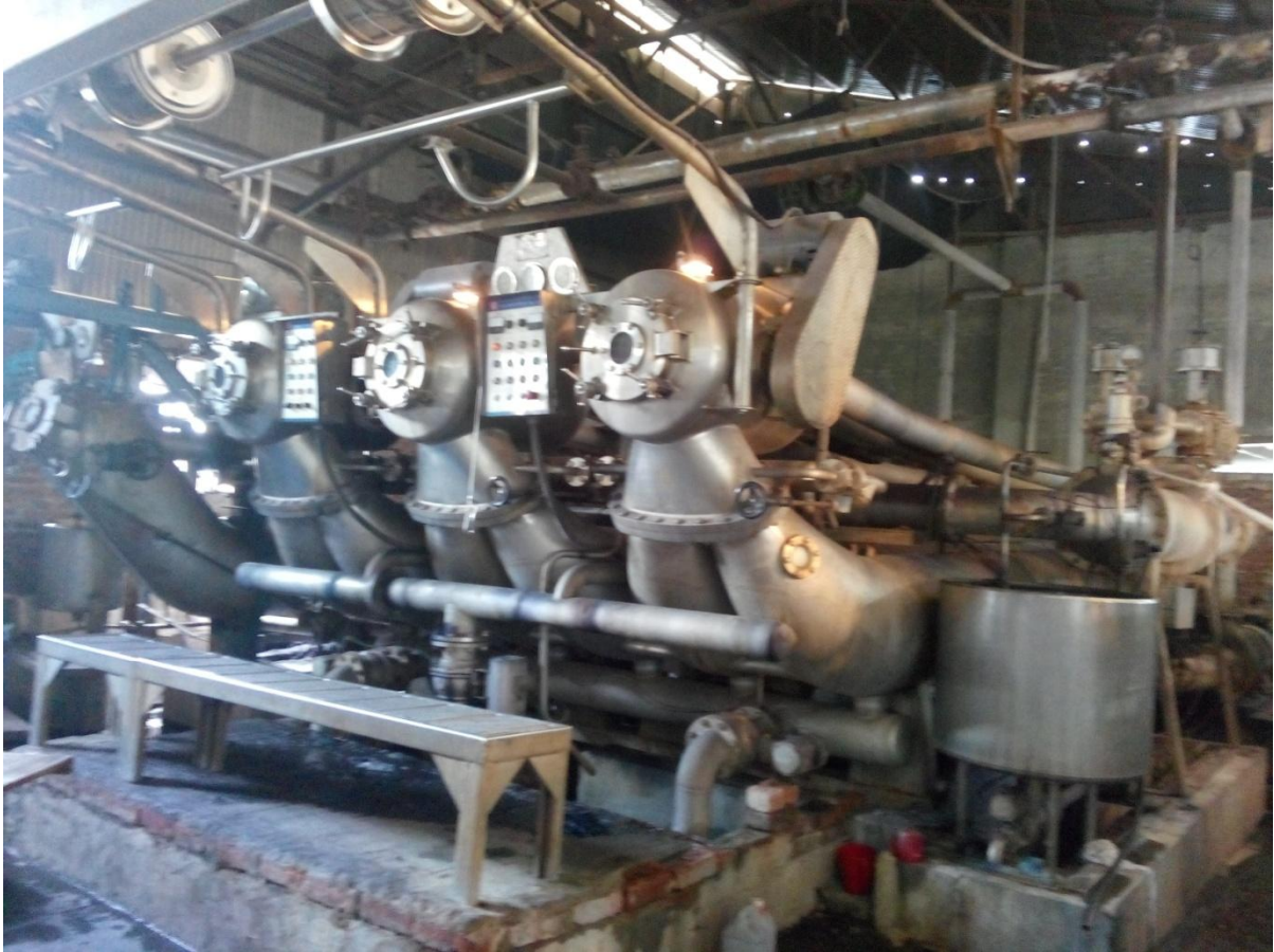
Figure No 05: Pictorial view of Jet dyeing Machine.
