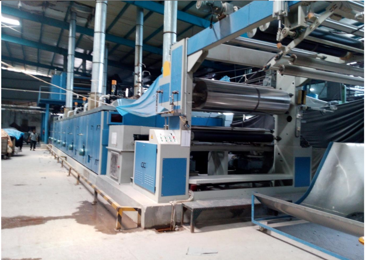
Figure No 09: Pictorial view of Stenter Machine.
