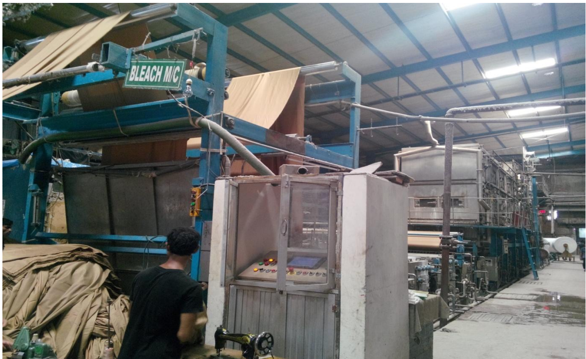
Figure 02: Pictorial view of one Bath Scouring and Bleaching Machine.
