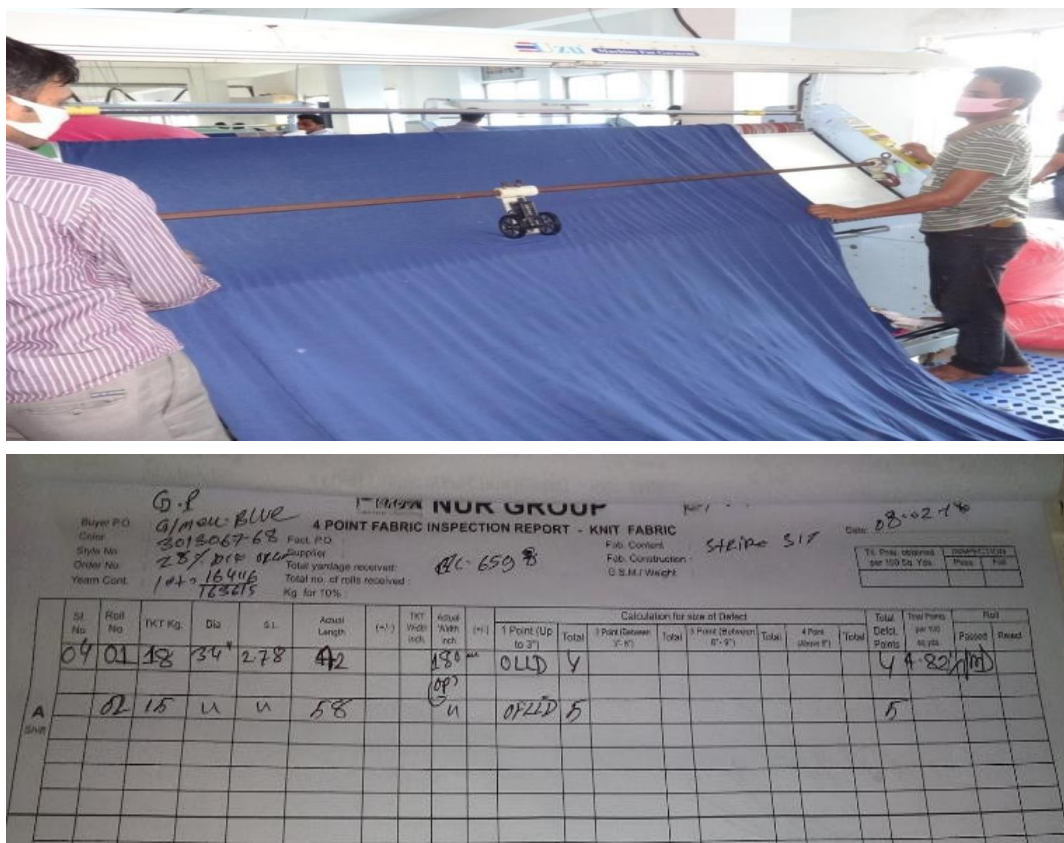
Fig: 2 Inspection 4-Points System:
