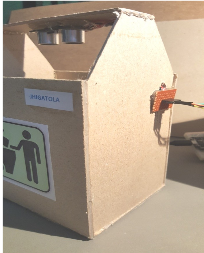
Fig-4.3: A smart dustbin with integrated ultrasonic sensor.
