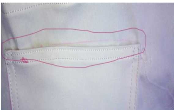
Figure 3.5.5: Uneven Lock in Tuck
