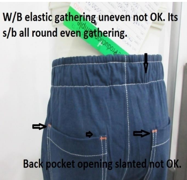
Fig 3.13 Defect Of PO. 10035284
