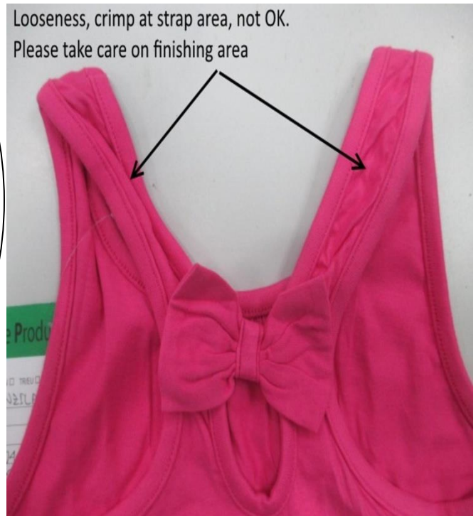
Fig 3.55 Defect of PO 10035277
