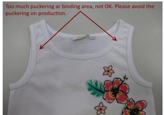
Fig 3.24 Defect of PO 10035283
