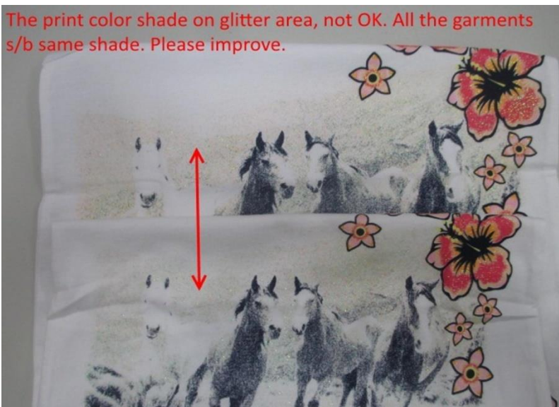
Fig 3.23 Defect of PO 10035283
