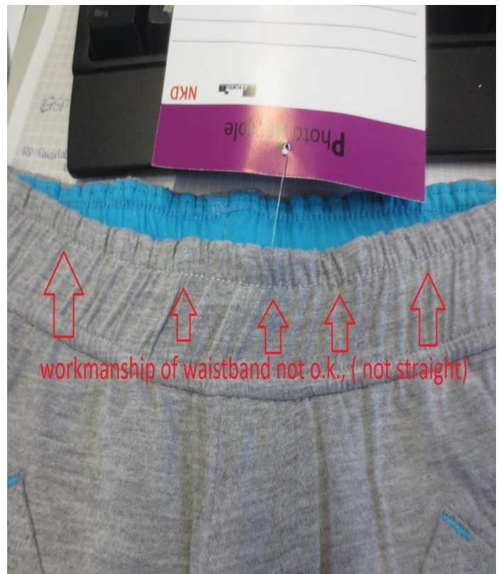
Fig 3.80 Defect of PO 10034328
