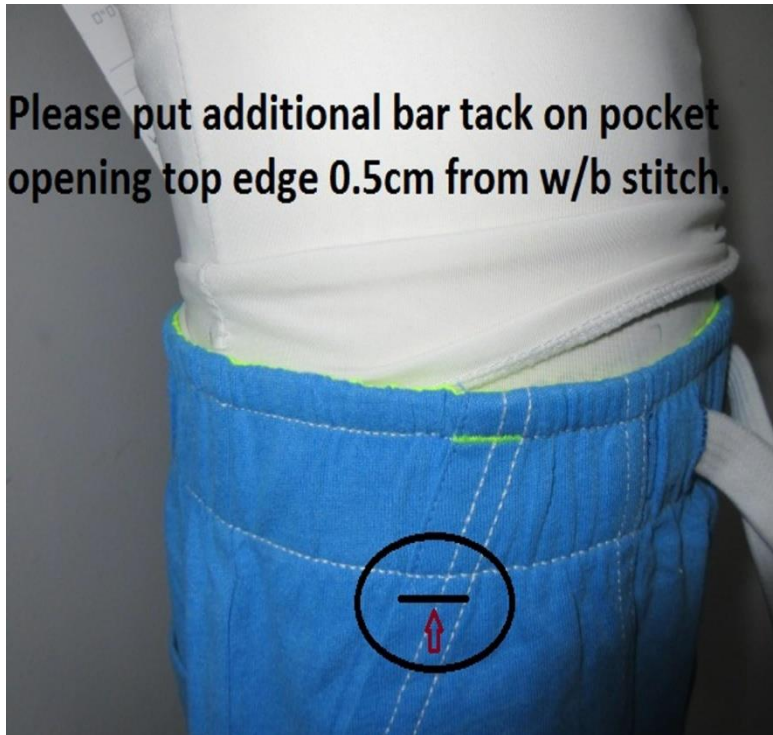
Fig 3.27 Defect of PO 10035316
