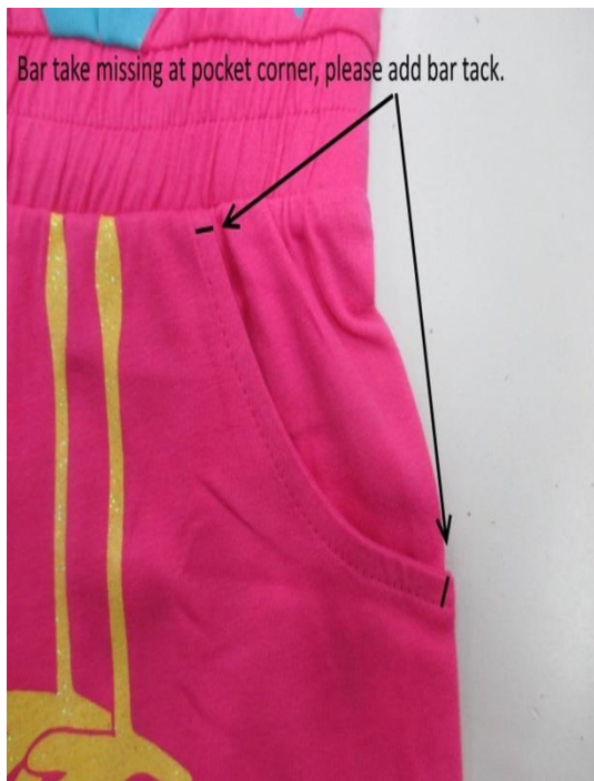
Fig 3.54 Defect of PO 10035277
