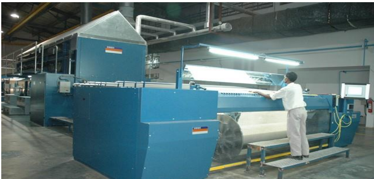
Figure 8 BENINGER Sizing Machine
