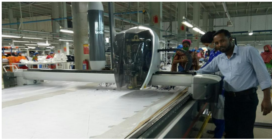
Fig 12: Fabric cut by auto cutter machine
