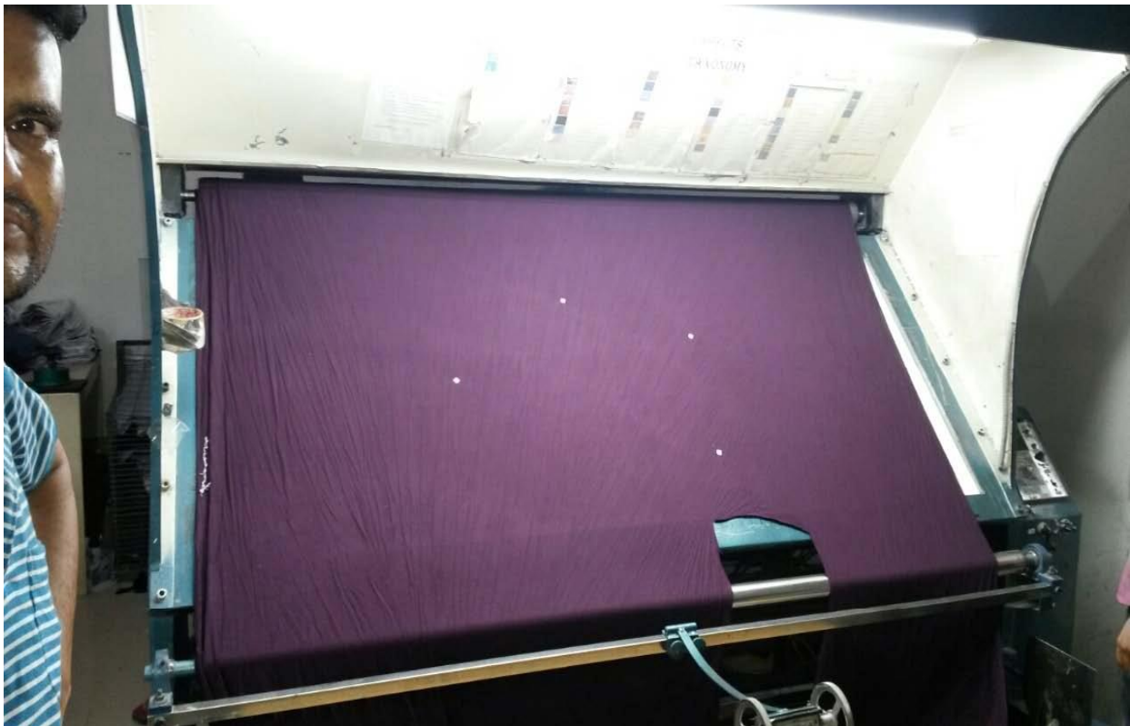
Fig: 4- point system inspection
