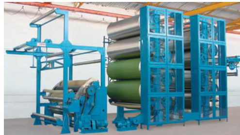
Figure 2.7: Cylinder Drying Machine
