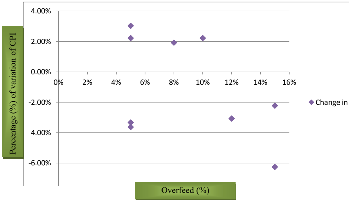
Figure 4.6: Correlation between overfeed% and change of CPI percentage (%)
