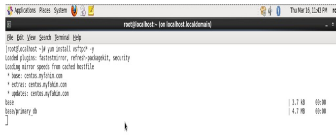
Figure 4.14: yum Server Installation
