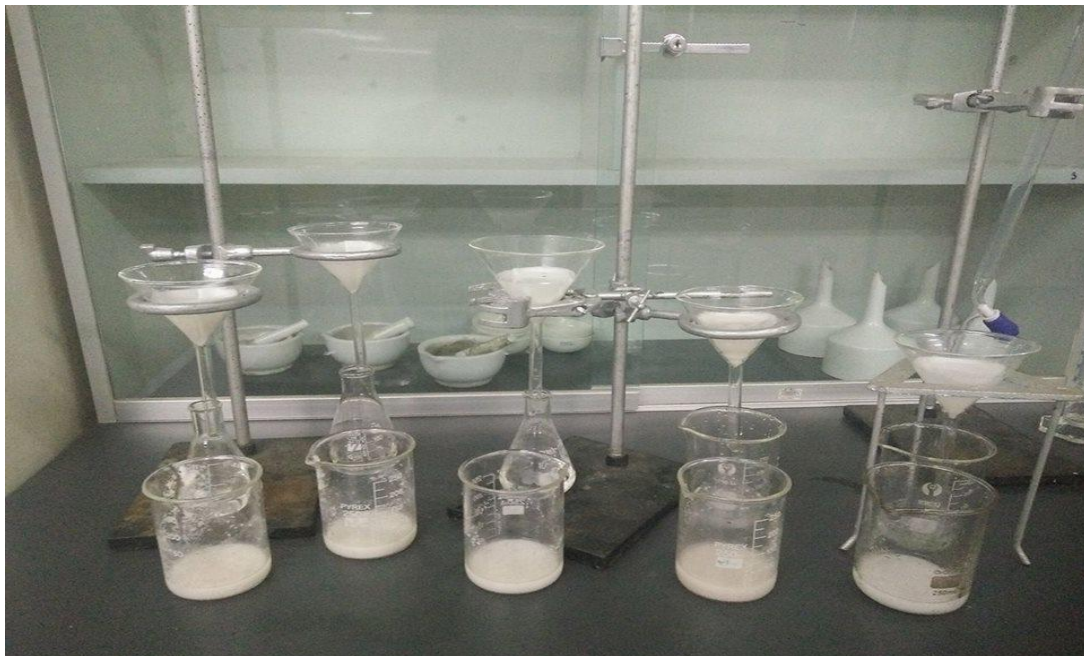
Figure 10: Filtration of fish flesh after add TCA
