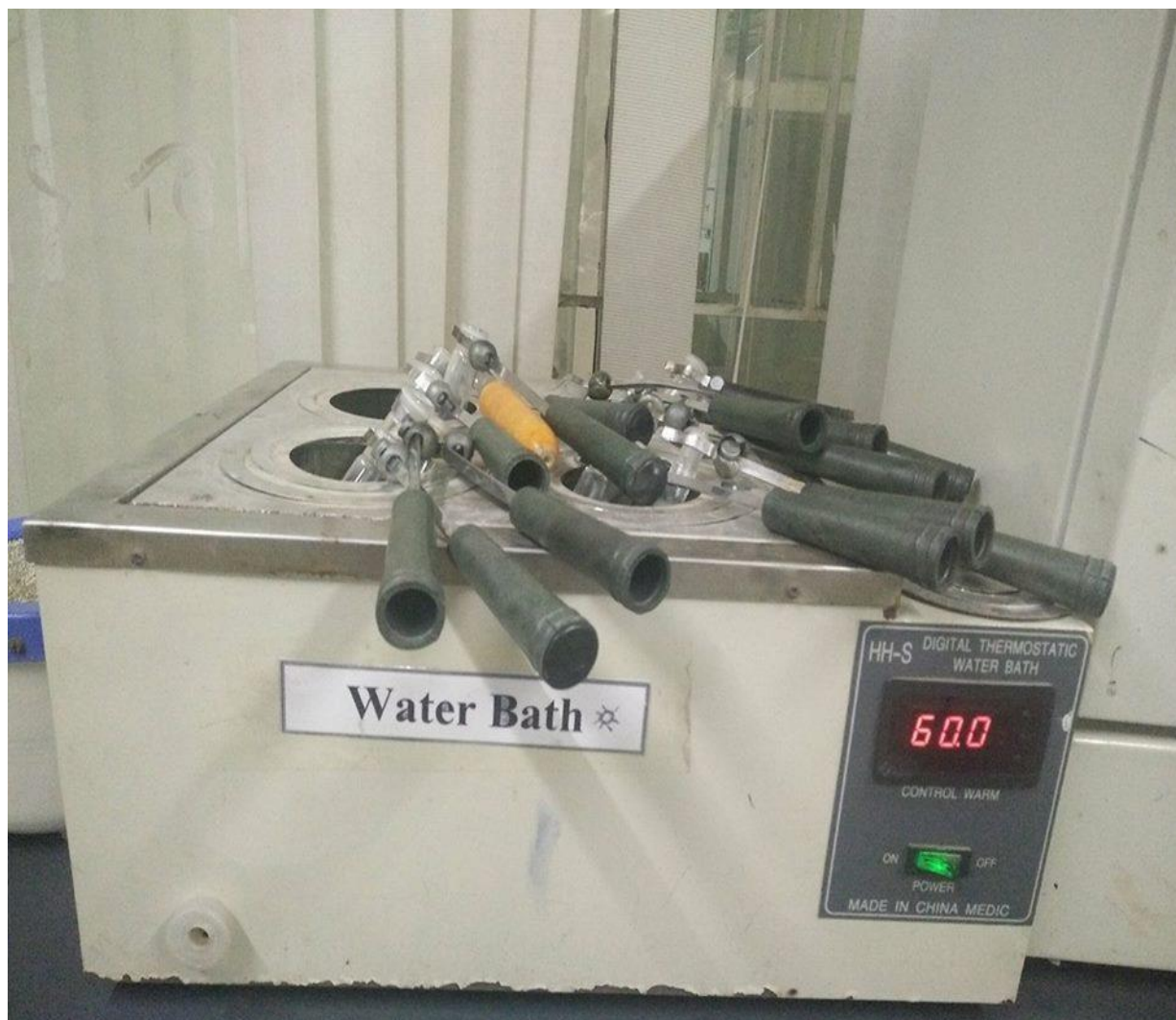
Figure 11: Filtrate of sample heat in water bath with Nash reagent
