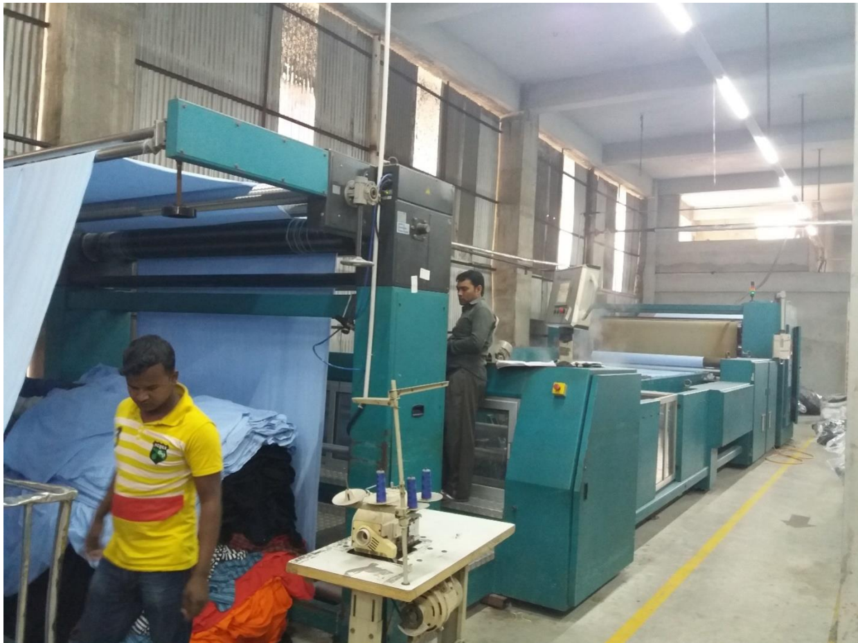
Fig: 3.2.13 Compactor Machine
