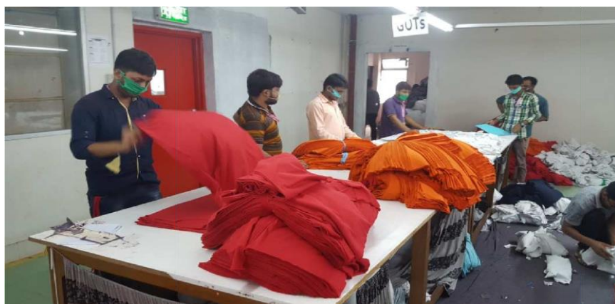
Fig: 3.3.13 Fabric Inspection after cutting
