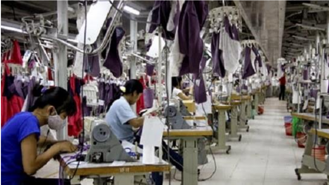
Fig 2.12.7.1 Line layout in UPS system
