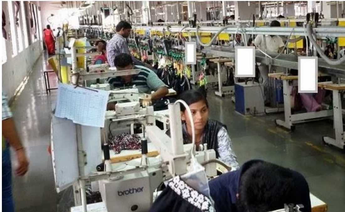
Fig 2.12.3.1 Straight line layout with overhead material transportation.
