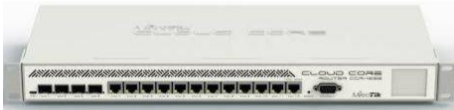
Figure 4.20: MikroTik Cloud Core Router
