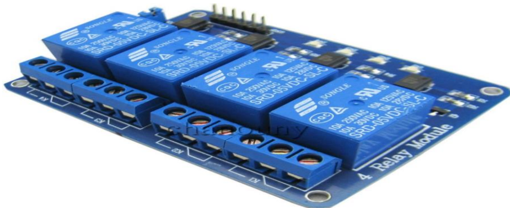
Figure: 4.9 Relay Shield
