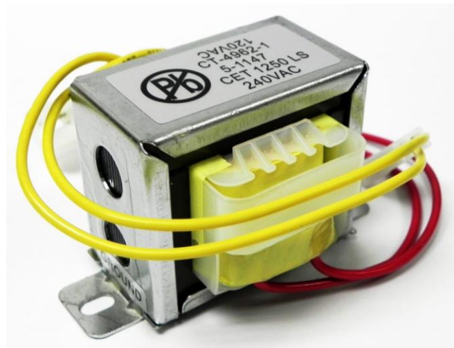
Figure: 4.10 Step-down Transformer
