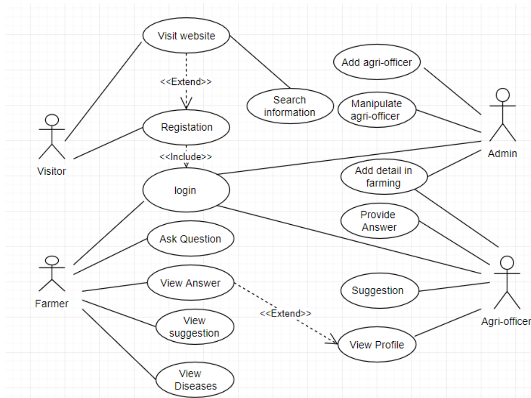
Figure 3.3.1:Smart farming use case Diagram
