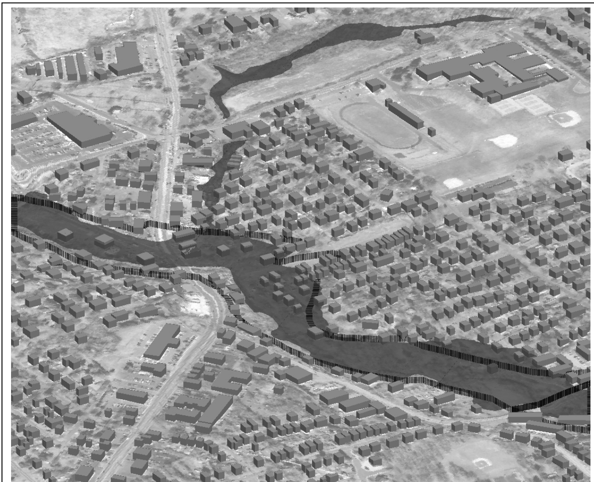
Figure 2: A 3D GIS simulation showing differences between the existing (shown as outline) and new (shown as solid areas) floodplain boundaries.
