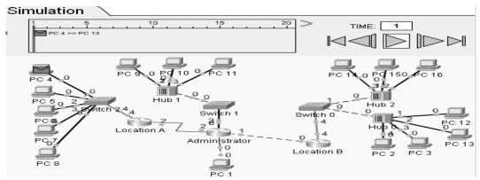
Fig. 3 Data has been sent to PC 13 from PC 4
