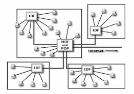
Fig. 2 Extended Star Topology in a Multi-Building Campus
