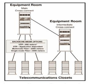
Fig. 1 Backbone media option of Telecommunications closet
