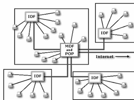
Fig. 2 Extended Star Topology in a Multi-Building Campus
