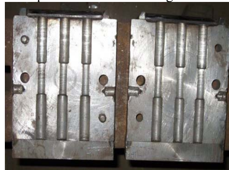
Fig.4: Tensile Specimen Permanent Mould
