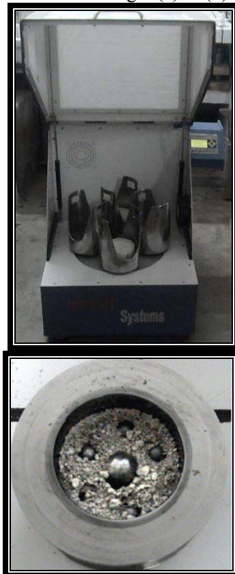
Fig.1: (a) Planetary High Energy Ball Mill (b) Mixing Jar loaded with milling balls and SiC
