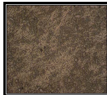
Fig.6: (c) Optical microstructure of A356 matrix reinforced with 0.5Wt% of micro SiC particles (125µm) at 200x magnification.
