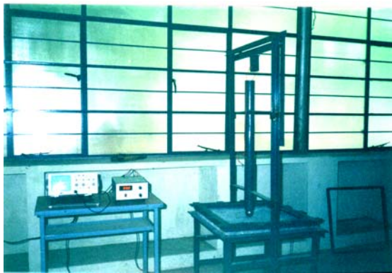
Fig. 1 (b): Drop Weight Impact Testing Machine
