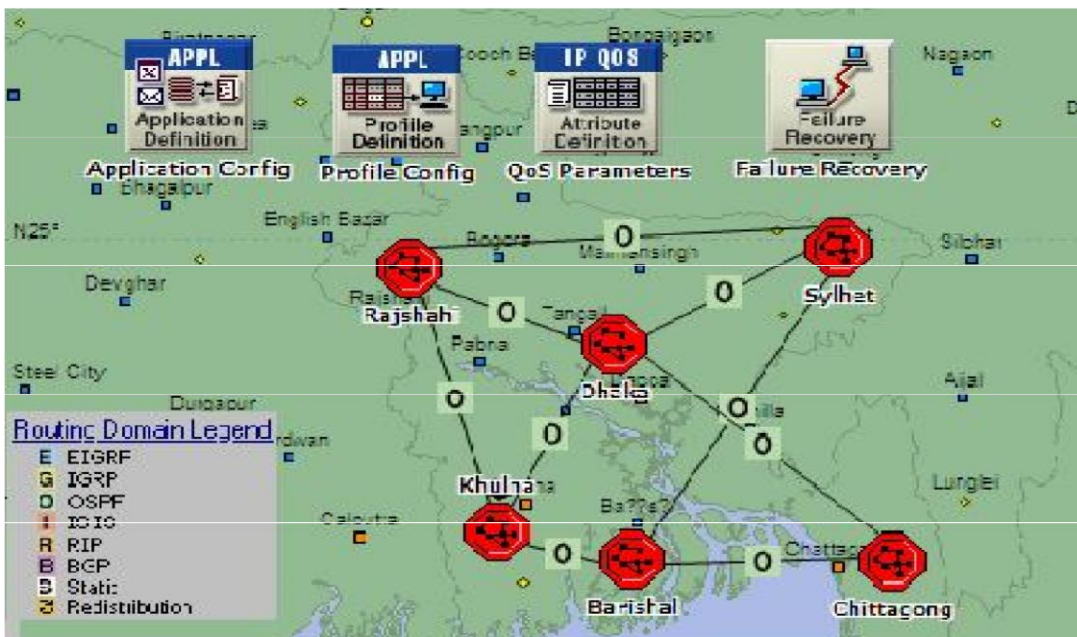
Figure 5.5: Network model for OSPF
