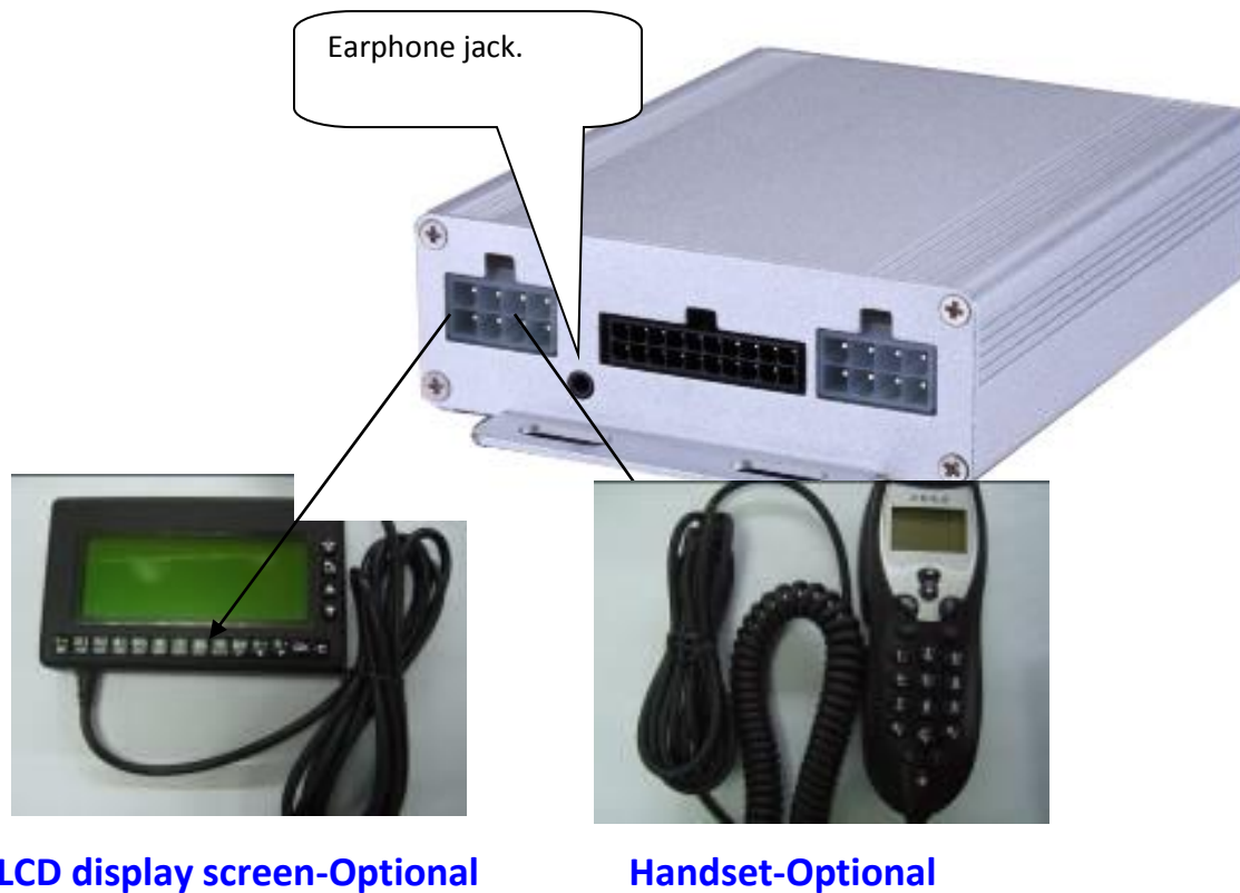
Figure 5.1: Host Tracker with LCD Display and Handset
