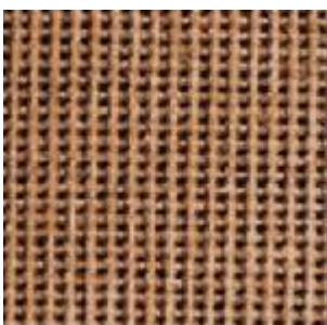
Fig: Jute carpet backing fabric
