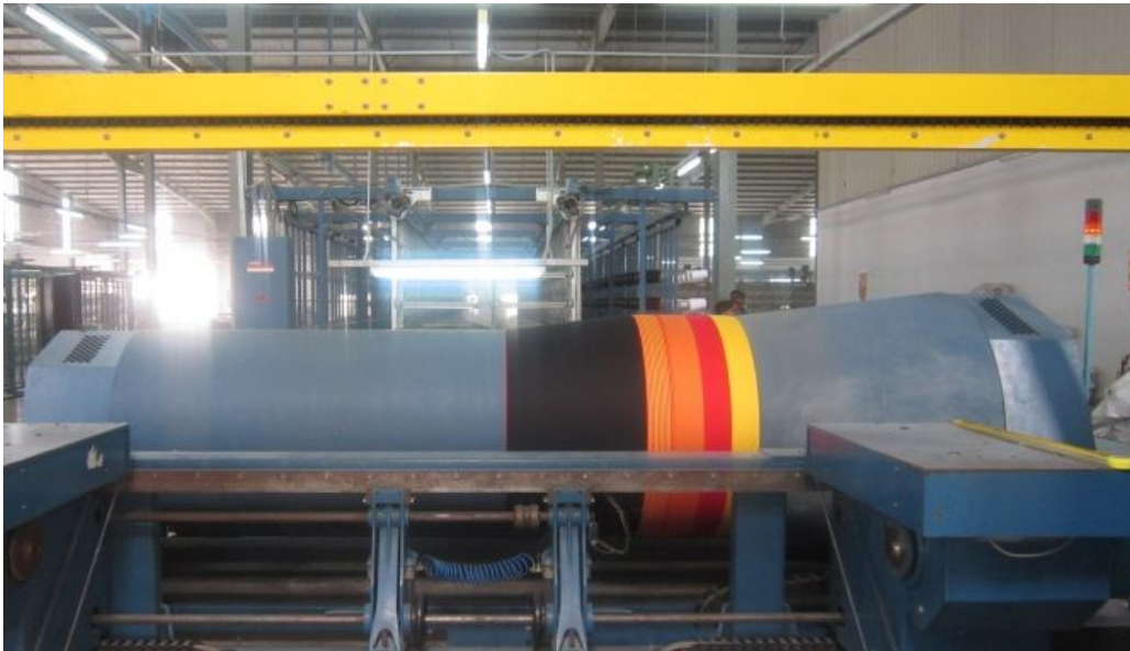
Fig – 6: Sectional Warping Machine from the front
