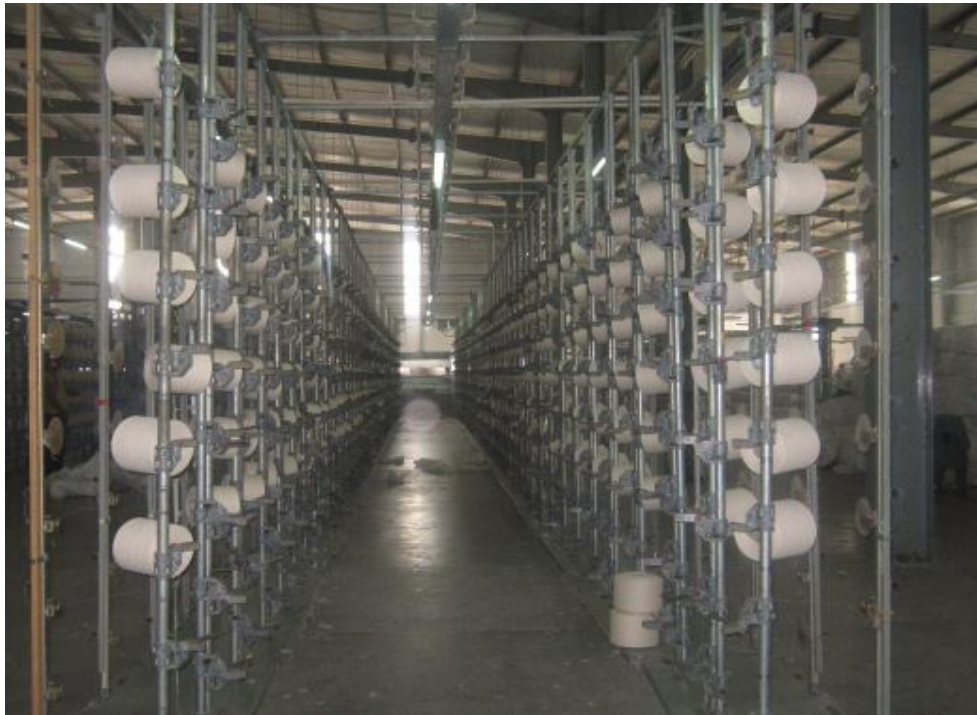
Fig – 5: Creel behind the Direct Warping Machine available in TFL
